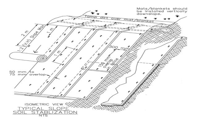
Figure 2. Erosion control blanket
