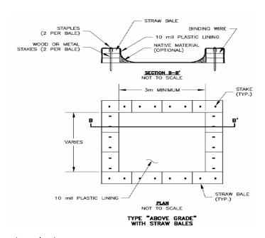
Figure 6. Above grade concrete washout
