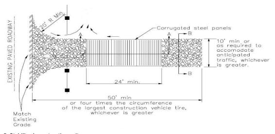
Figure 5. Stabilized construction exit
