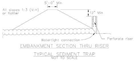
Figure 4. Pipe outlet sediment trap
